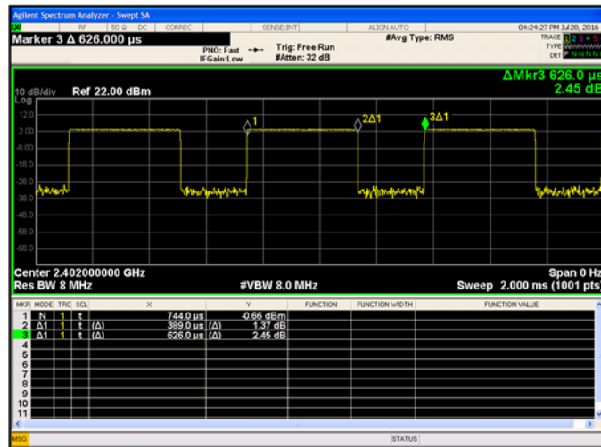
Figure 9-1. Duty Cycle 2402MHz (Ch.0)
