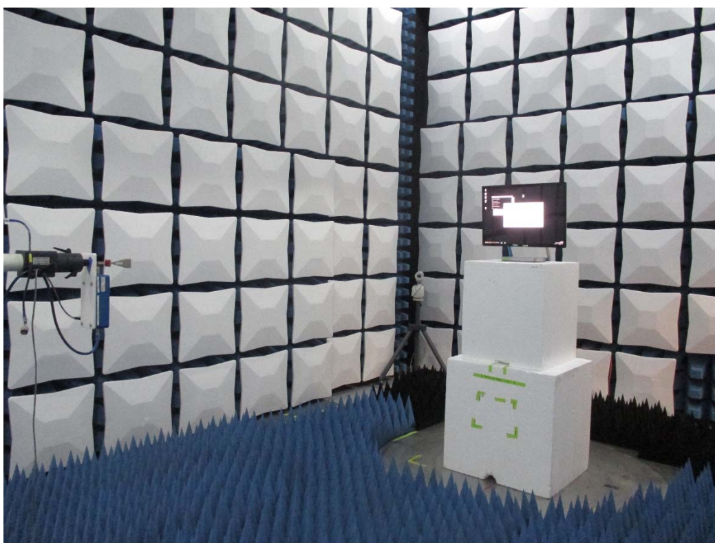
Fig.4 Radiated Spurious Emissions (18-26.5GHz) Test Site2
