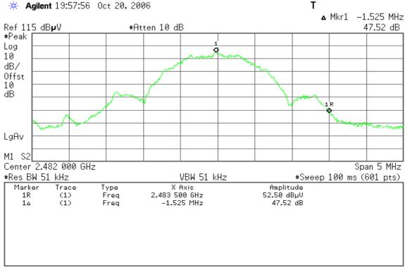
Delta marker at 1% of span = 47.52dB
