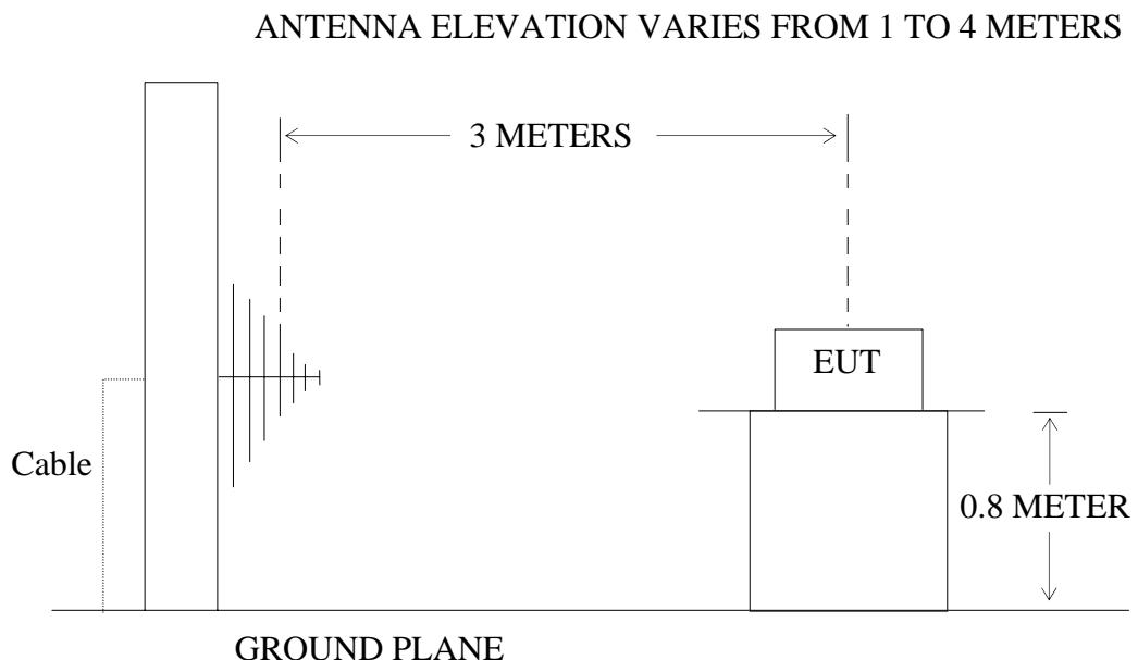
(EUT: Weather Station Transmitter)
