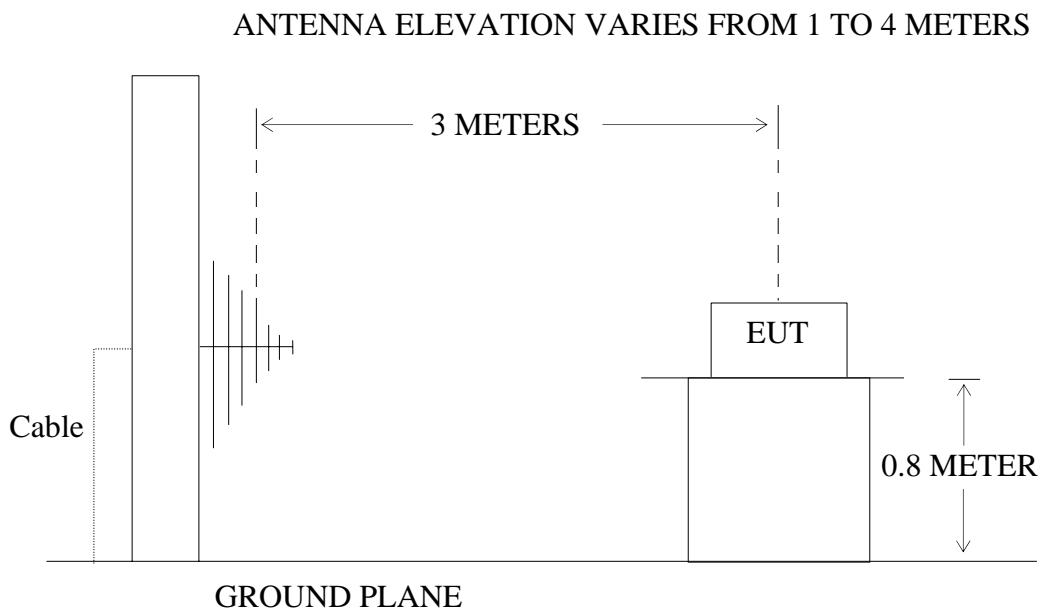
(EUT: Weather Station Transmitter)
