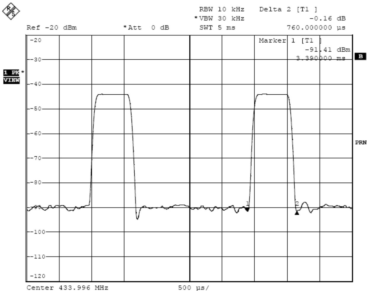
The graph shows the duration of 'on' signal. From marker 1 to marker 2, duration is 0.76ms.
