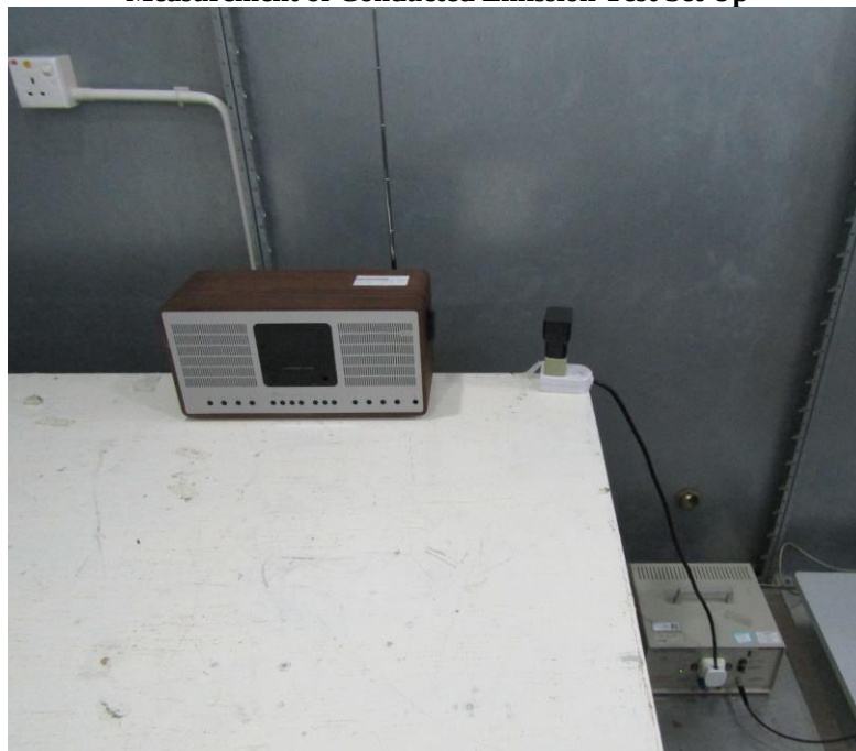
Measurement of Conducted Emission Test Set Up
