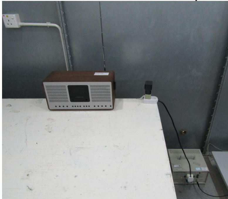
Measurement of Conducted Emission Test Set Up
