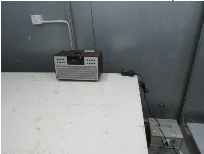
Measurement of Conducted Emission Test Set Up
