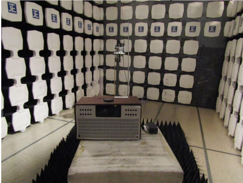
Measurement of Conducted Emission Test Set Up
