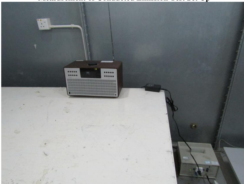
Measurement of Conducted Emission Test Set Up
