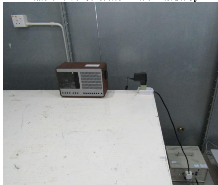
Measurement of Conducted Emission Test Set Up
