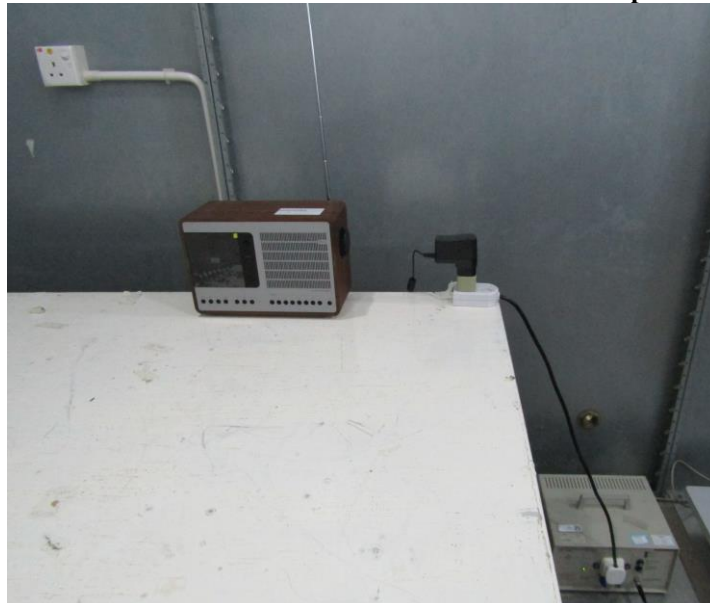
Measurement of Conducted Emission Test Set Up
