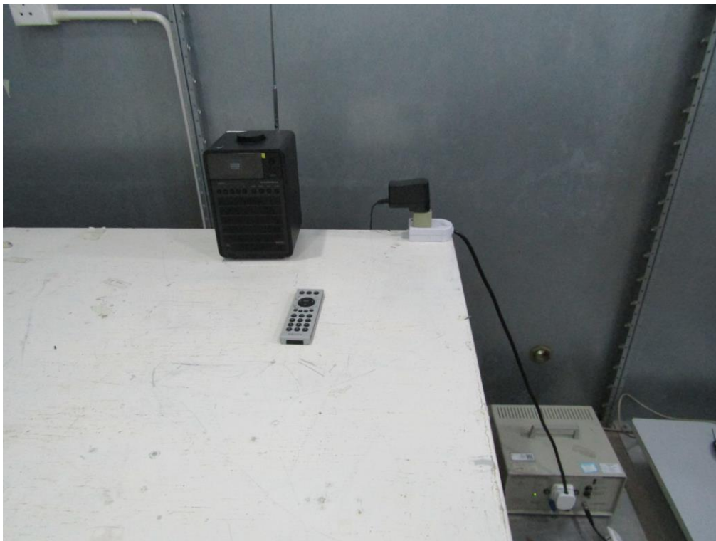
Measurement of Conducted Emission Test Set Up
