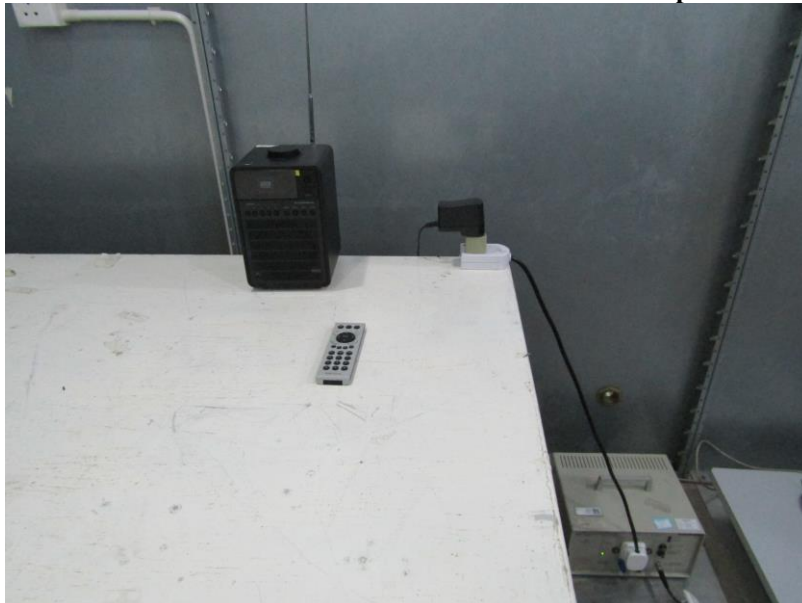
Measurement of Conducted Emission Test Set Up
