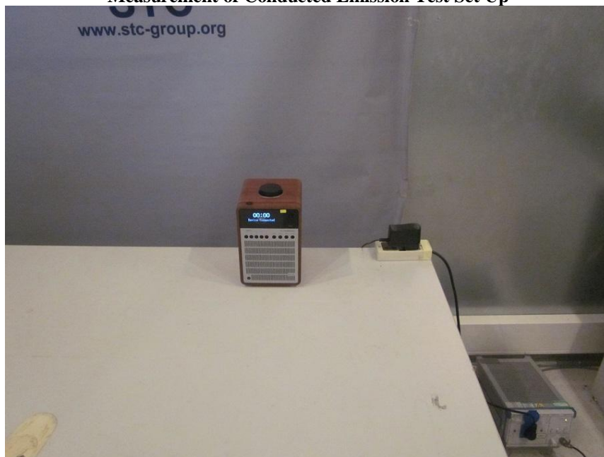
Measurement of Conducted Emission Test Set Up
