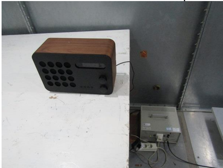
Measurement of Conducted Emission Test Set Up
