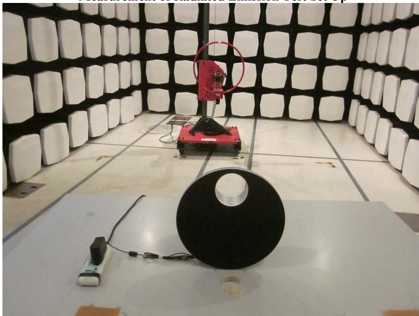
Measurement of Radiated Emission Test Set Up
