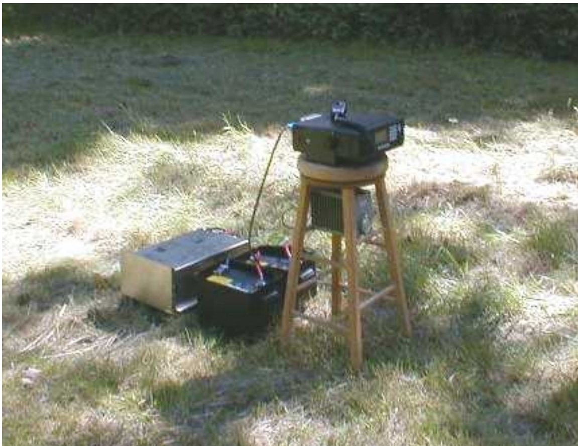
FIGURE 4 TRANSCEIVER ON TURNTABLE WITH BATTERY SYSTEM
