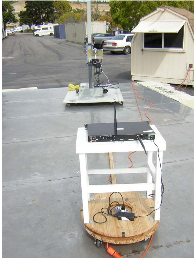
Photograph 2. Radiated Emissions Test Configuration
