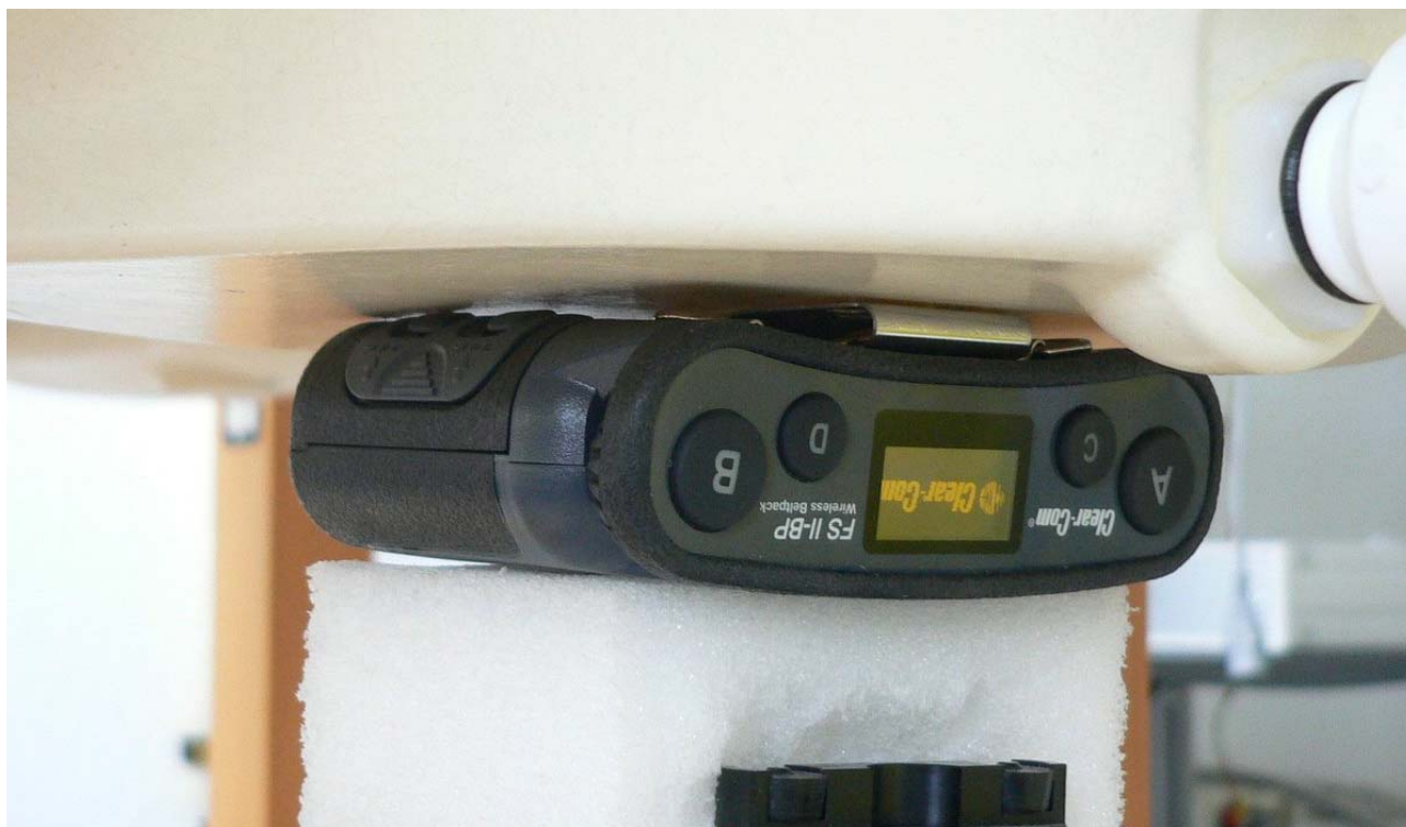
Fig. 10: Body worn configuration for Clear-Com BP1G9, position 2, back side towards the phantom, 0 mm distance.
