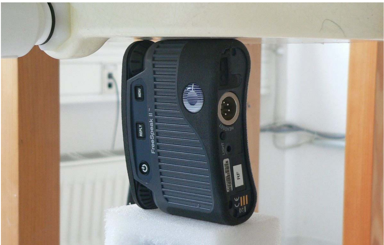
Fig. 14: Body worn configuration for Clear-Com BP1G9, position 6, right edge towards the phantom, 0 mm distance.
