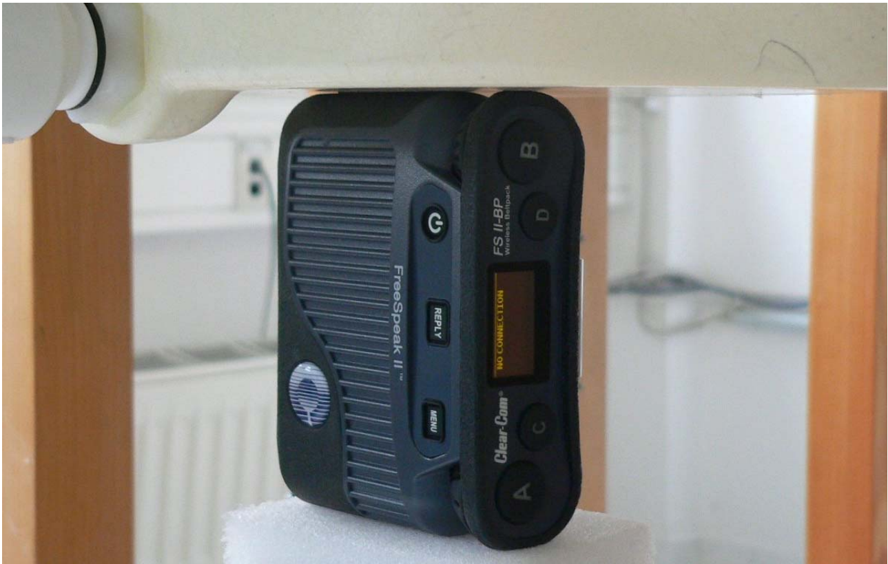
Fig. 13: Body worn configuration for Clear-Com BP1G9, position 5, left edge towards the phantom, 0 mm distance.
