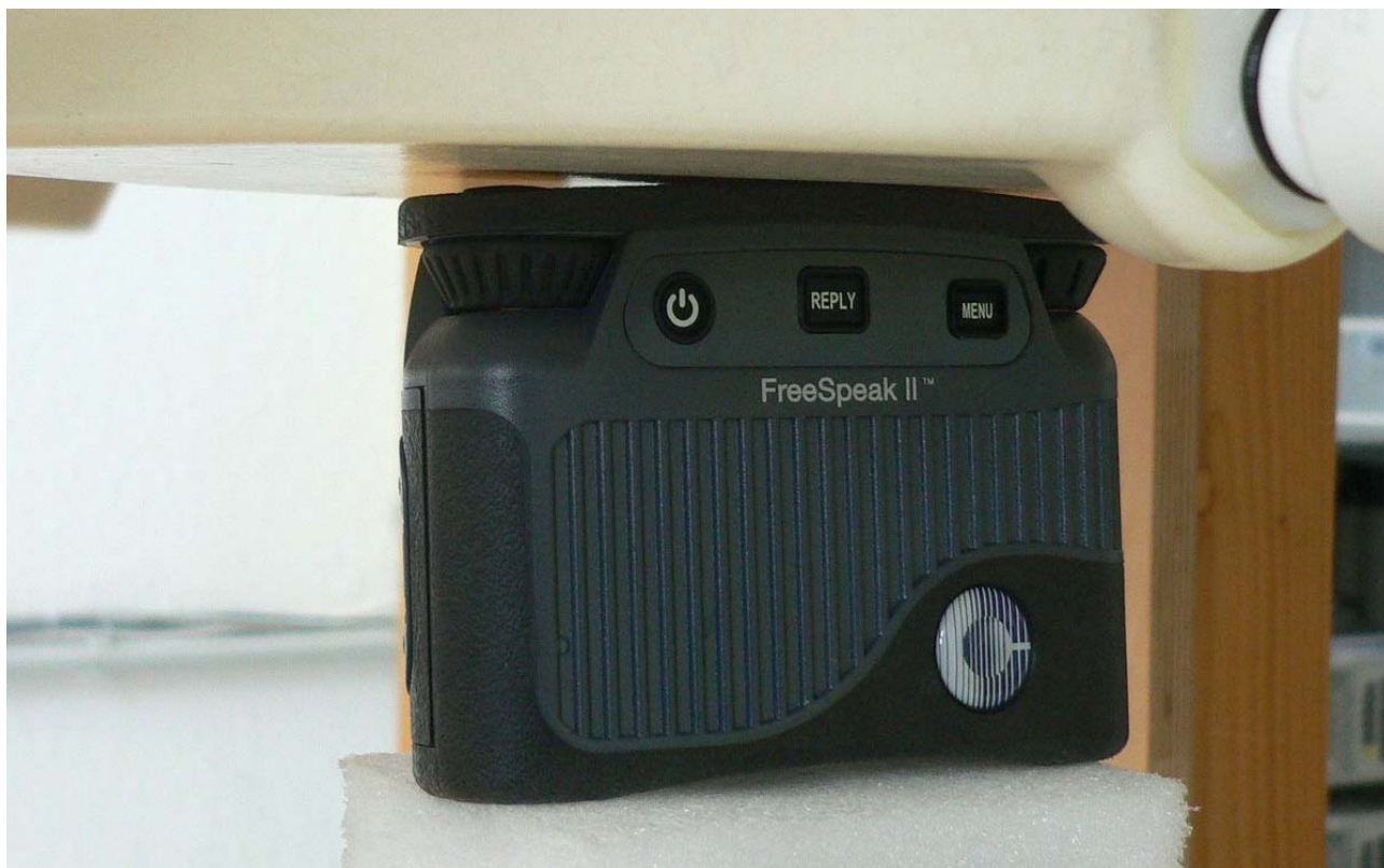
Fig. 11: Body worn configuration for Clear-Com BP1G9, position 3, top edge towards the phantom, 0 mm distance.
