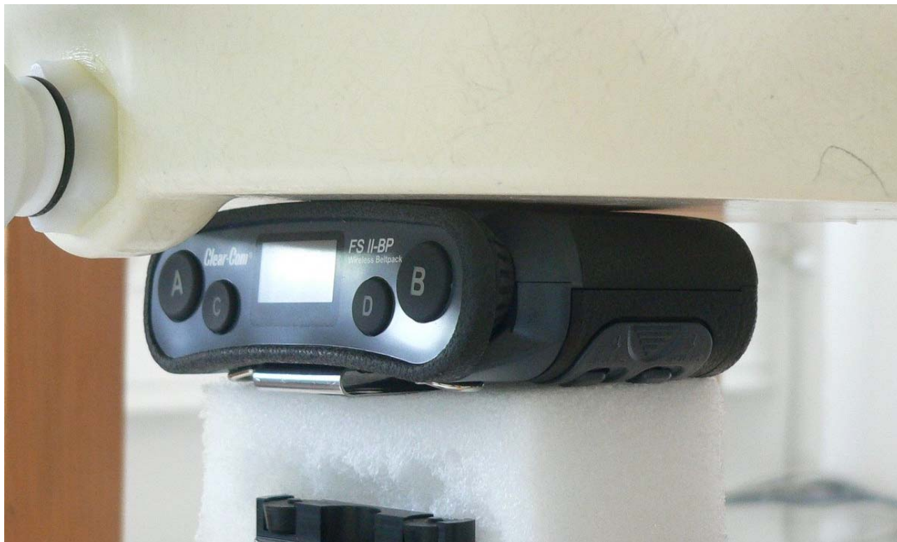
Fig. 9: Body worn configuration for Clear-Com BP1G9, position 1, front side towards the phantom, 0 mm distance.
