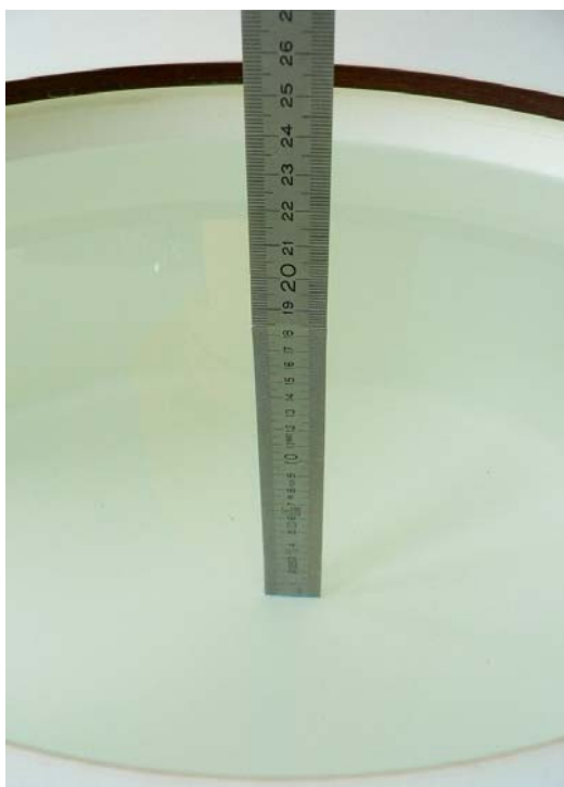
Fig. 15: Liquid depth for 1900 MHz Body worn measurements.
