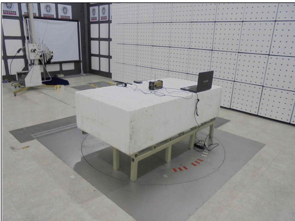
RADIATED EMISSION TEST (Mode B)
