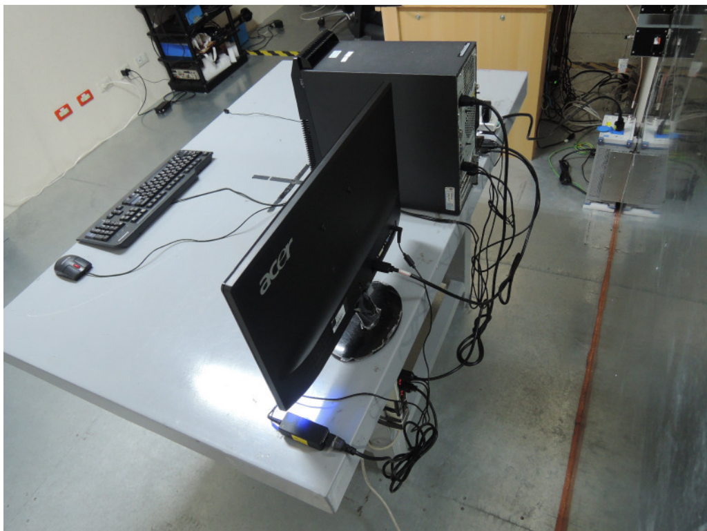
Photograph 5: Set-up for for Mains Conducted testing Back
