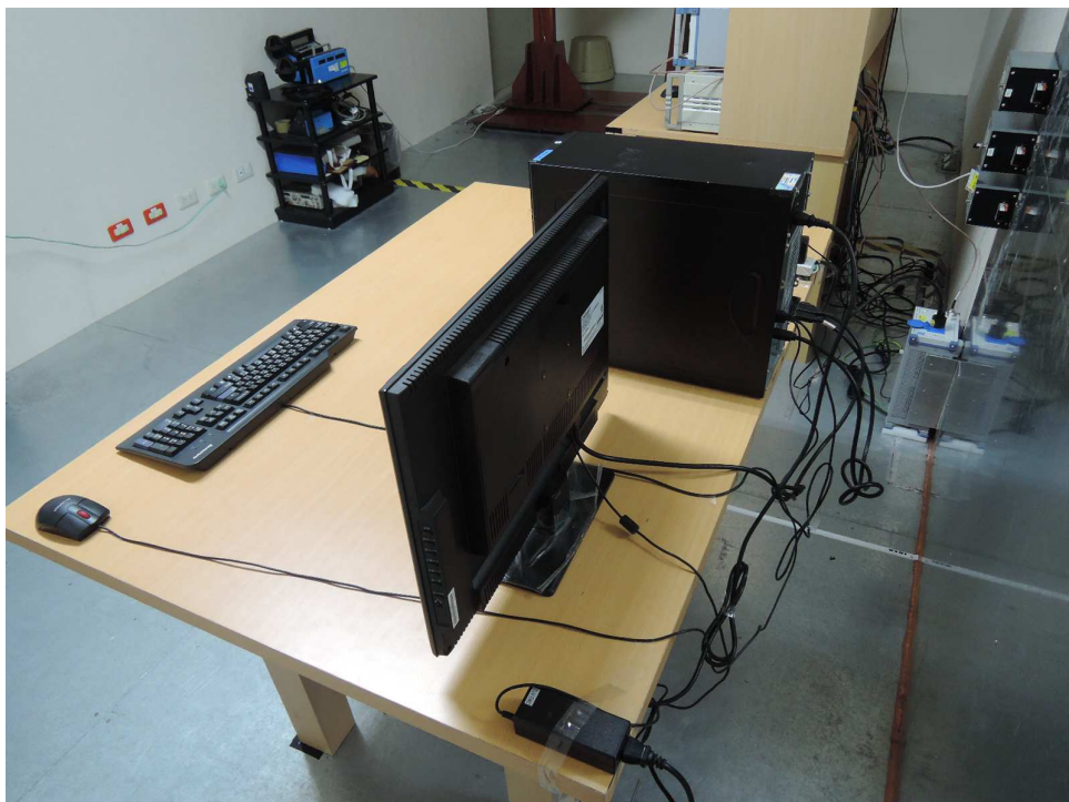
Photograph 5: Set-up for for Mains Conducted testing Back
