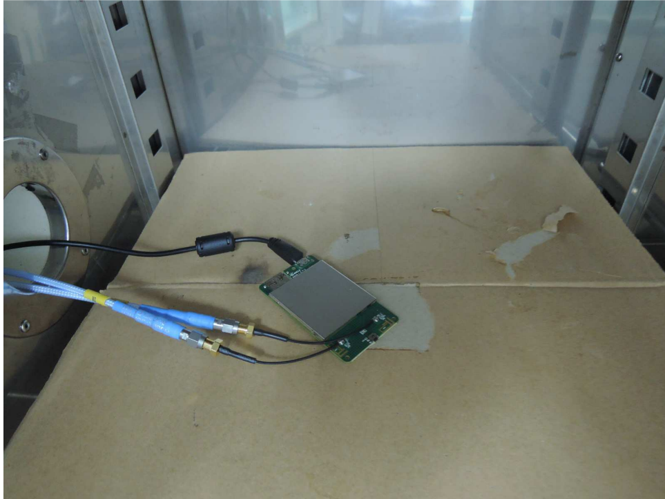
Photograph 4: Set-up for Conducted testing
