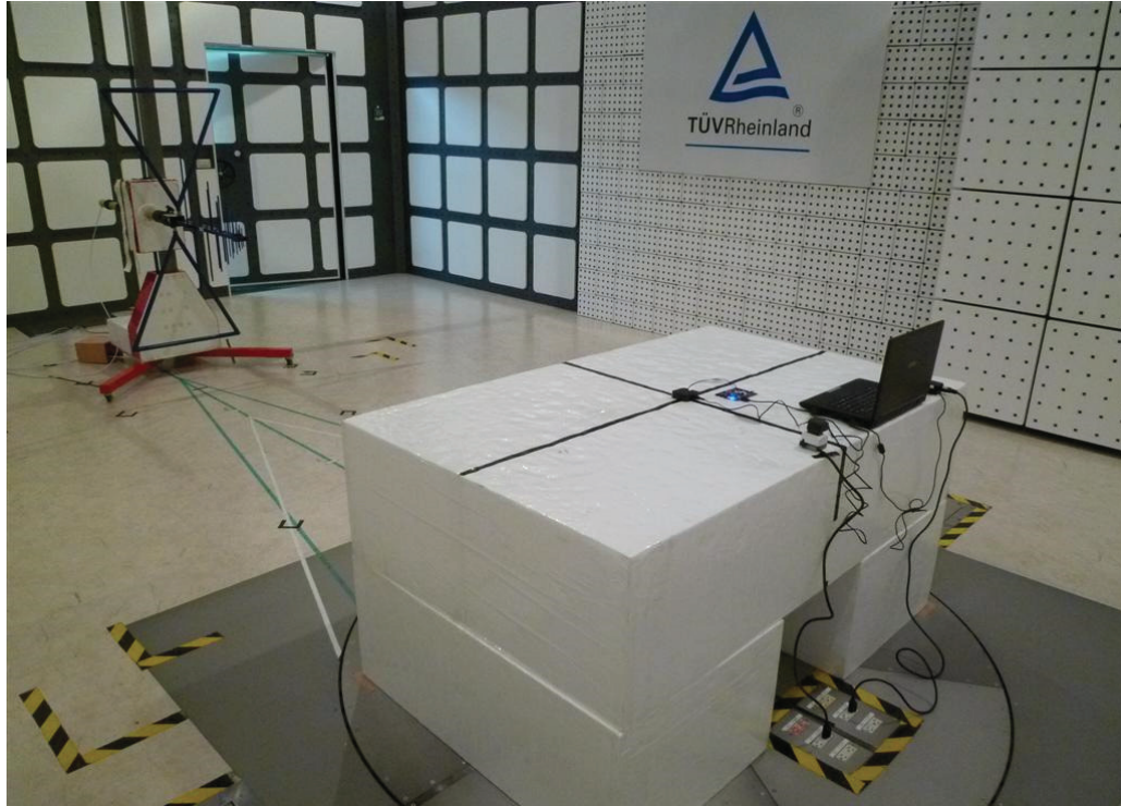
Photograph 2: Set-up for Spurious Emissions (Back View 1)
