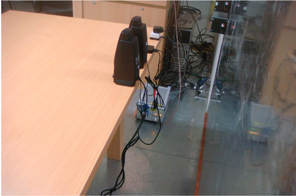
Photograph 5: Set-up for for Mains Conducted testing Back
