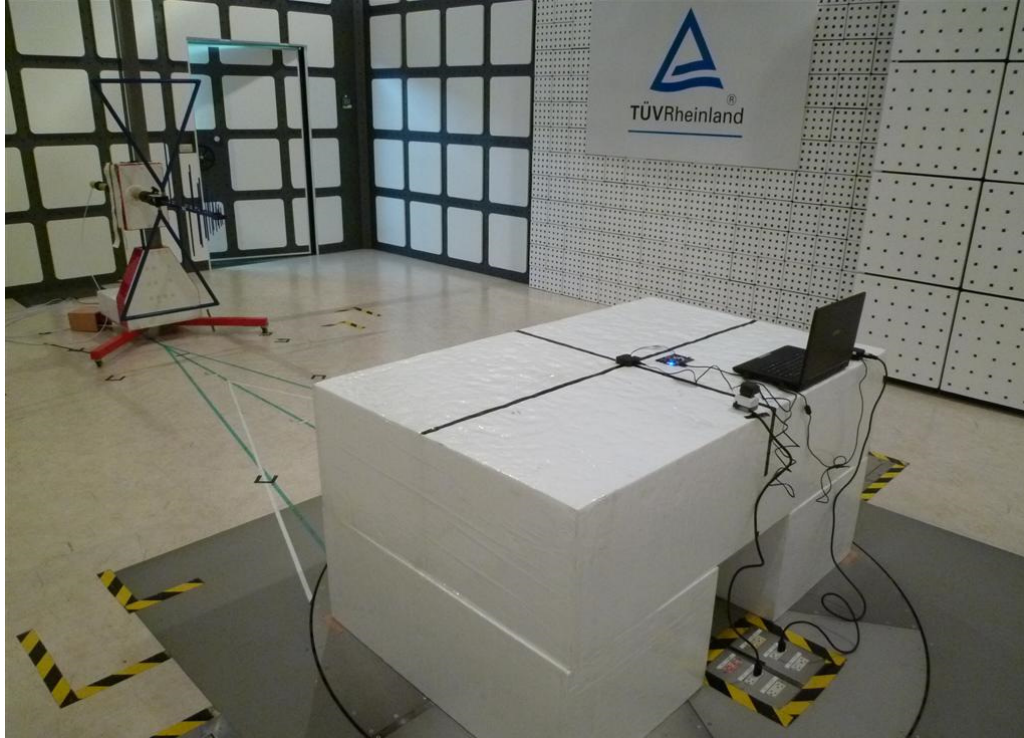
Photograph 2: Set-up for Spurious Emissions (Back View 1)
