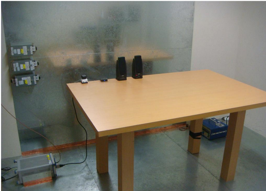
Photograph 6: Set-up for for Mains Conducted testing Front
