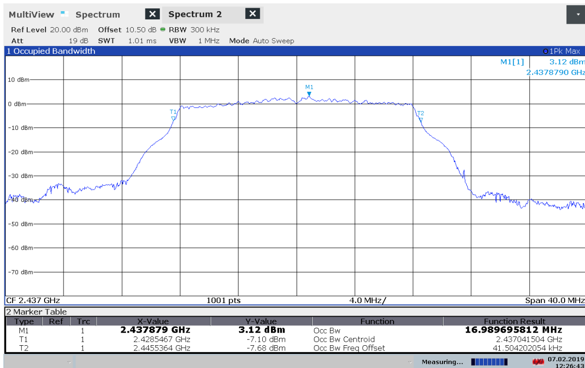
Occupied Bandwidth, 2437 MHz, 802.11g, 6Mbps
