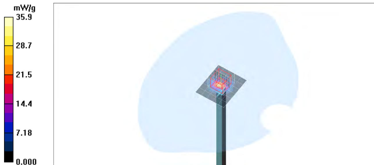
Plot. 19: SAR Verification Measurement 5800 MHz (on 19.03.2019), Body.
