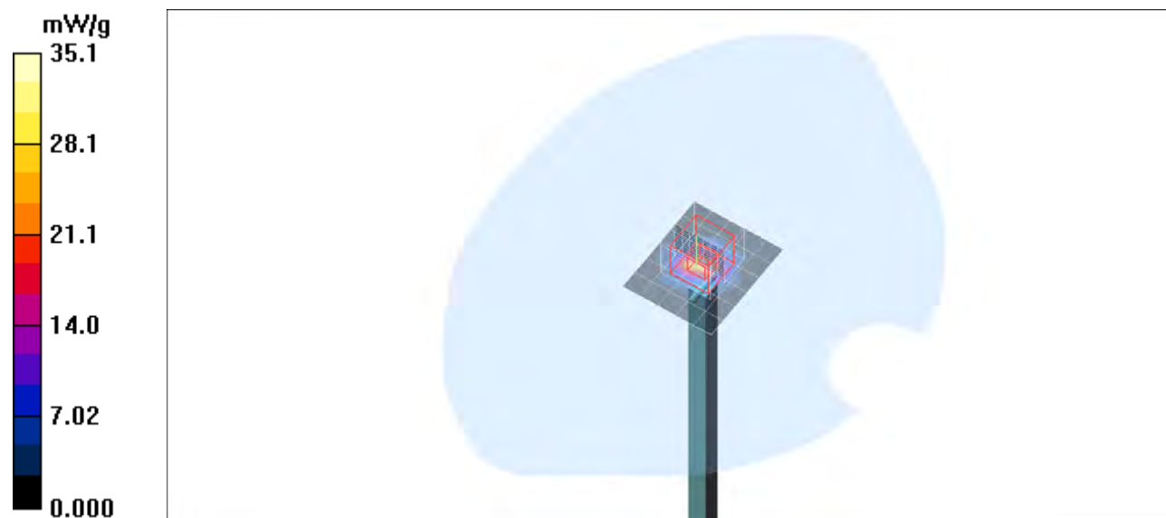
Plot. 12: SAR Verification Measurement 5250 MHz (on 01.04.2019), Head.
