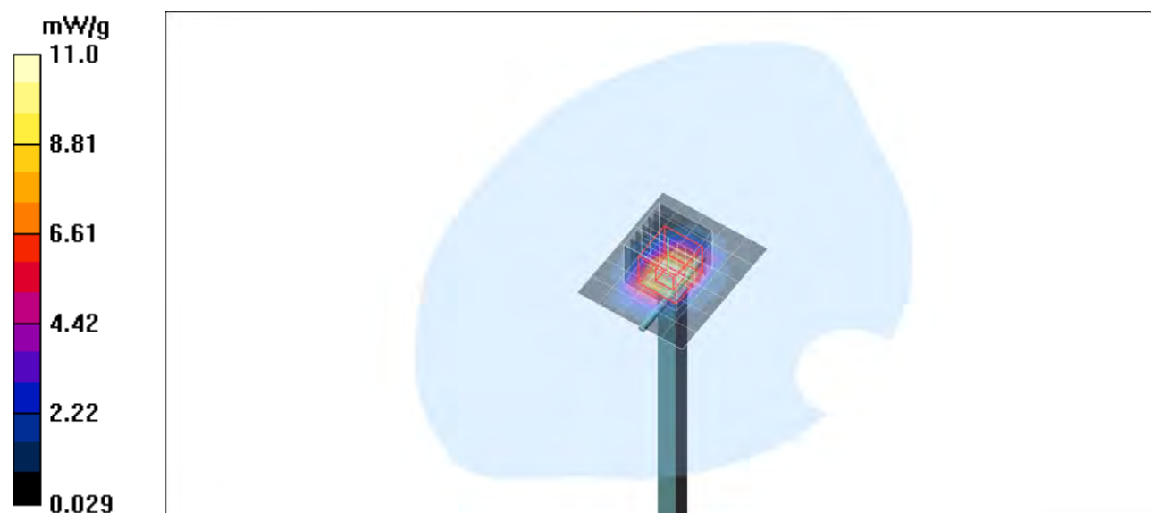
Plot. 15: SAR Verification Measurement 2450 MHz (on 16.05.2019 for BT), Body.
