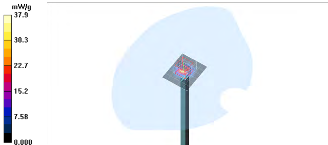
Plot. 18: SAR Verification Measurement 5600 MHz (on 19.03.2019), Body.
