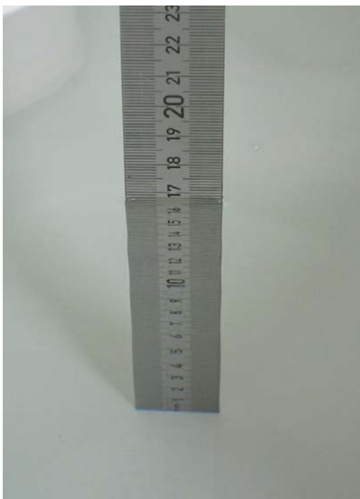
Fig. 47: Liquid depth for IEEE 802.11 b/n Body measurements
