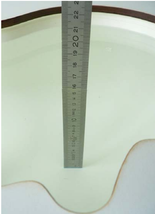
Fig. 45: Liquid depth for IEEE 802.11 b/n Head measurements
