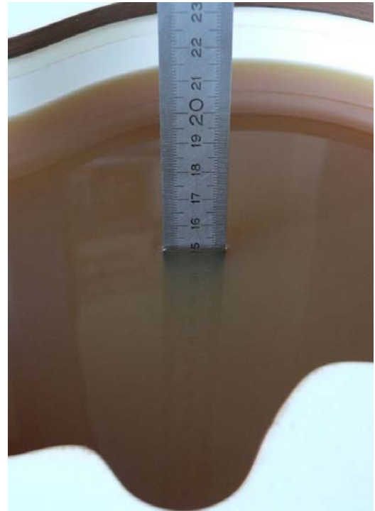
Fig. 46: Liquid depth for IEEE 802.11 a/n Head measurements
