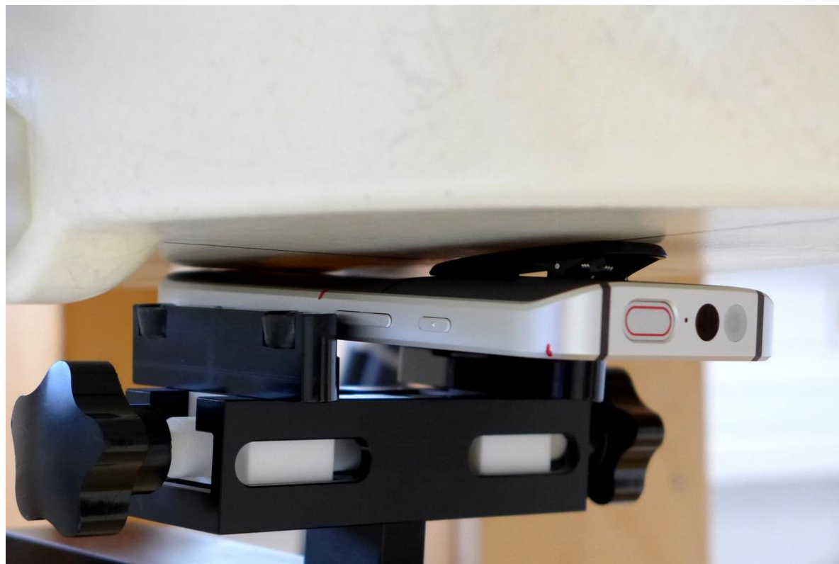
Pic. 11: Test position rear side of DUT towards the phantom, 0 mm gap, belt clip attached.
