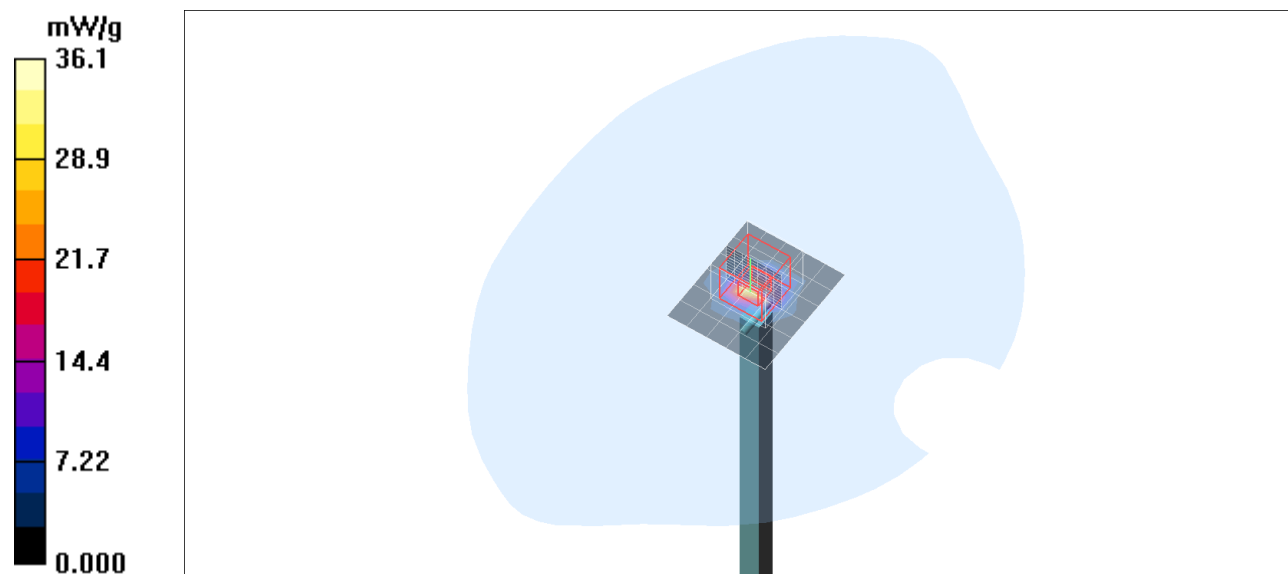
Plot. 17: SAR Verification Measurement 5250 MHz, Head, (July 9, 2020).
