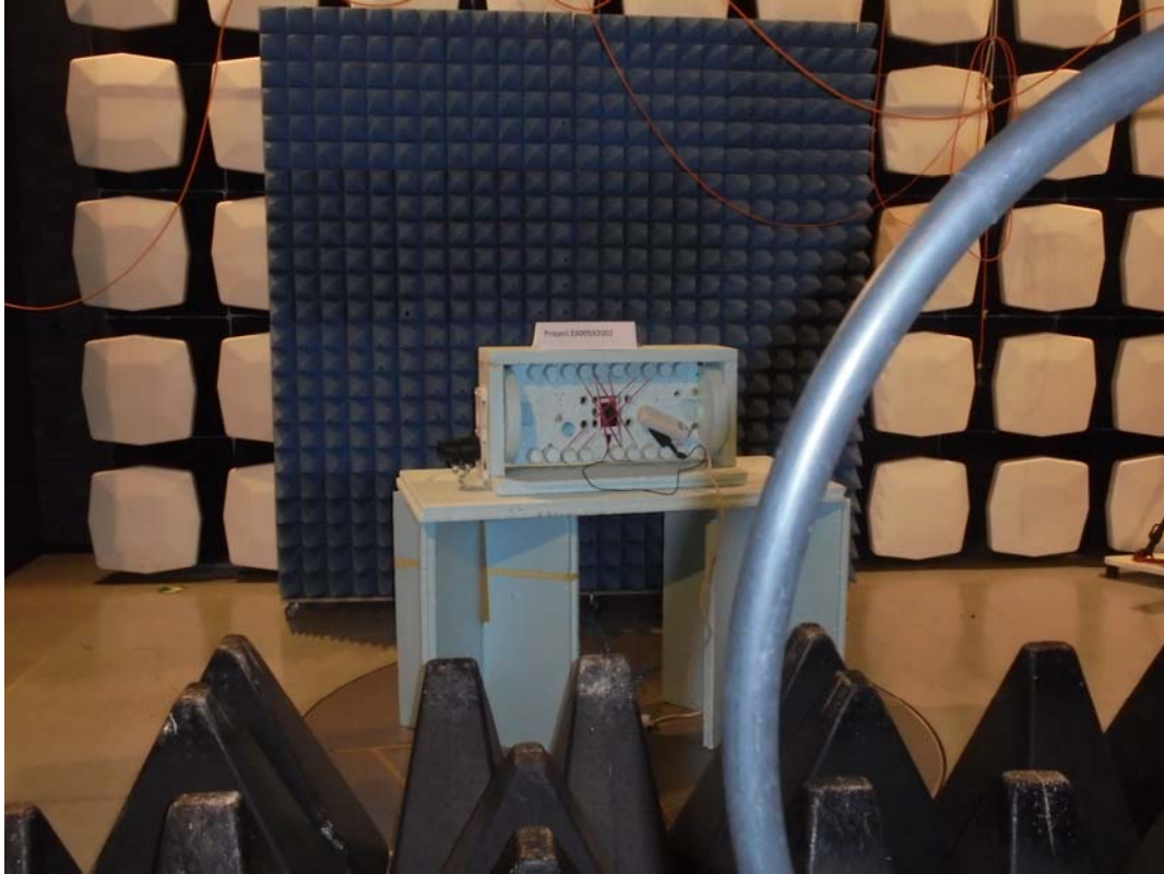
Test setup below 30MHz, long shot view
