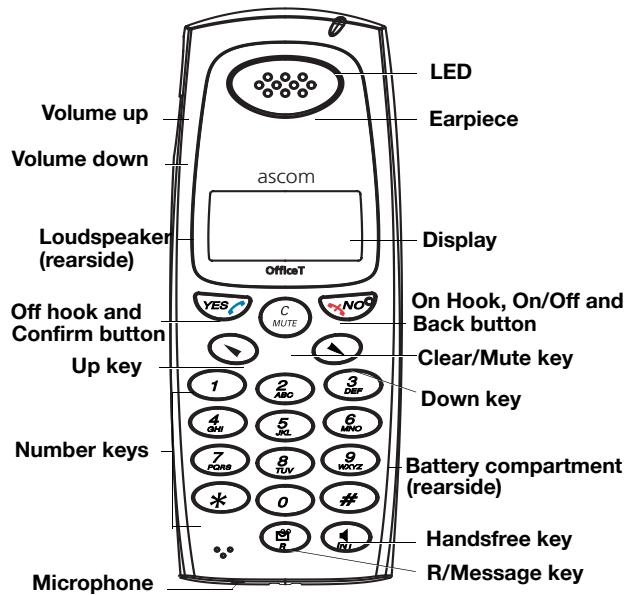
The lists below explains the use of the buttons and keys on the Cordless telephone.
