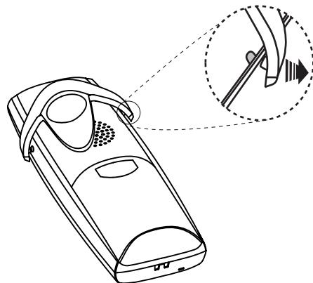
**Note:** To minimize wear and tear, we recommend that you do not remove the clip from the telephone too often.
