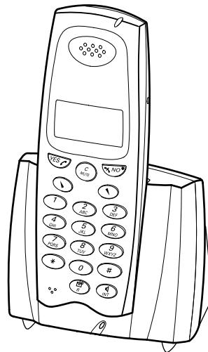
The battery is being charged when the lower green LED on the charger is on (and the “Battery icon” on the display flashes). If the battery is completely flat it can take a few minutes before the lower green LED on the charger comes on.
