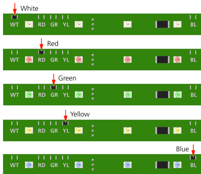
Figure 47. LED lamp boards: white, red, green, yellow and blue
