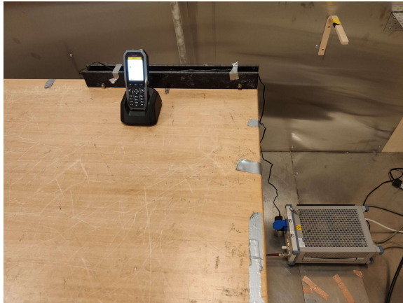
Power-Line Conducted Emissions
