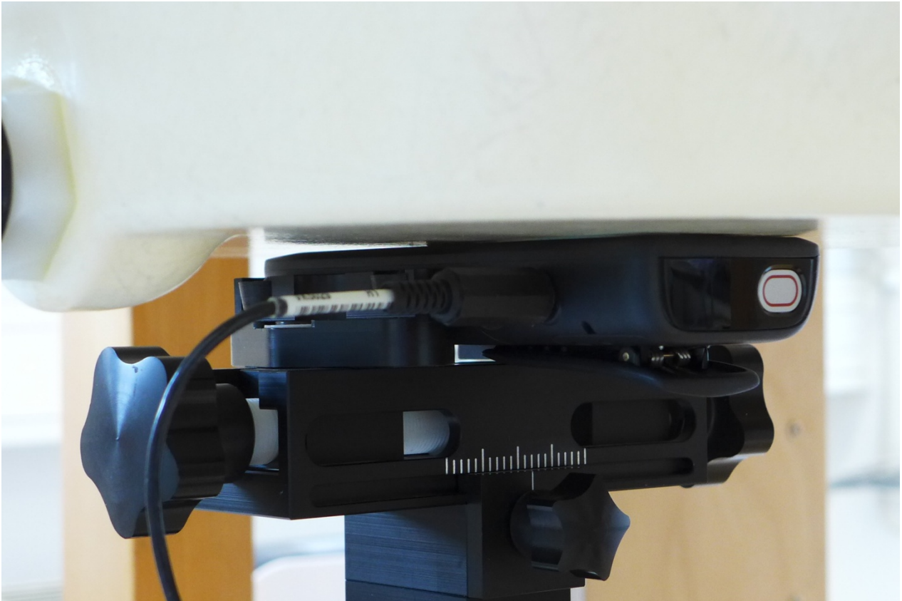
Fig. 19: Body worn configuration for DH7, front of the device towards the phantom, headset and belt clip attached, 0 mm distance.
