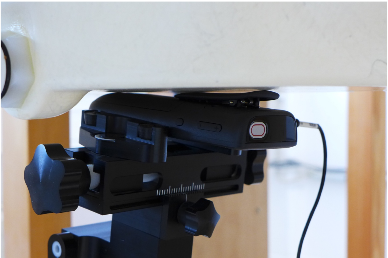
Fig. 20: Body worn configuration for DH7, back of the device towards the phantom, headset and belt clip attached, 0 mm distance.
