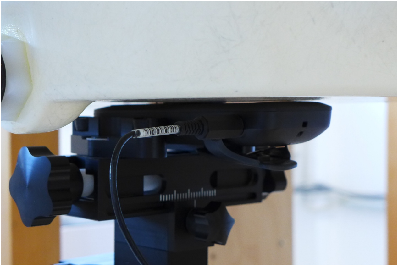
Fig. 19: Body worn configuration for DH6, front of the device towards the phantom, headset and belt clip attached, 0 mm distance.
