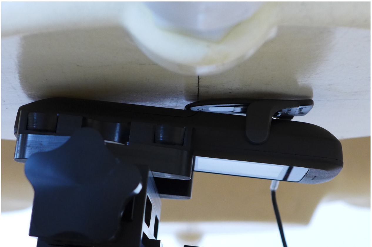
Fig. 20: Body worn configuration for DH6, back of the device towards the phantom, headset and belt clip attached, 0 mm distance.
