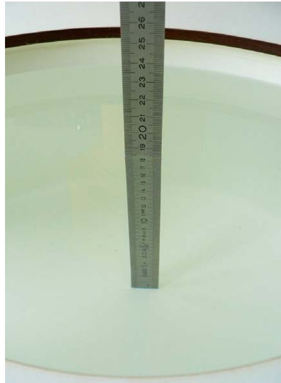
Fig. 22: Liquid depth for 1900 MHz Body worn measurements
