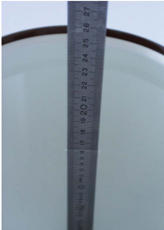
Fig. 21: Liquid depth for 1900 MHz Head measurements
