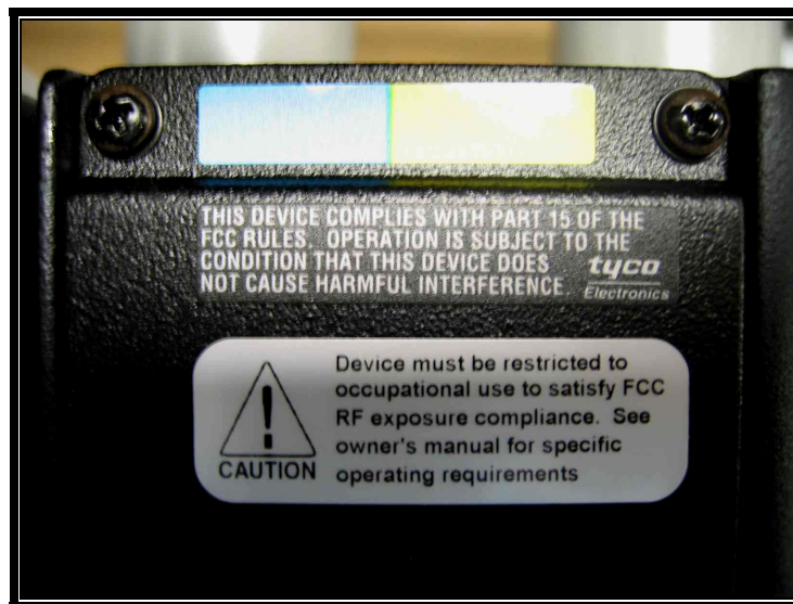
PHOTOGRAPH 2: PART 15 AND RF WARNING LABELS
