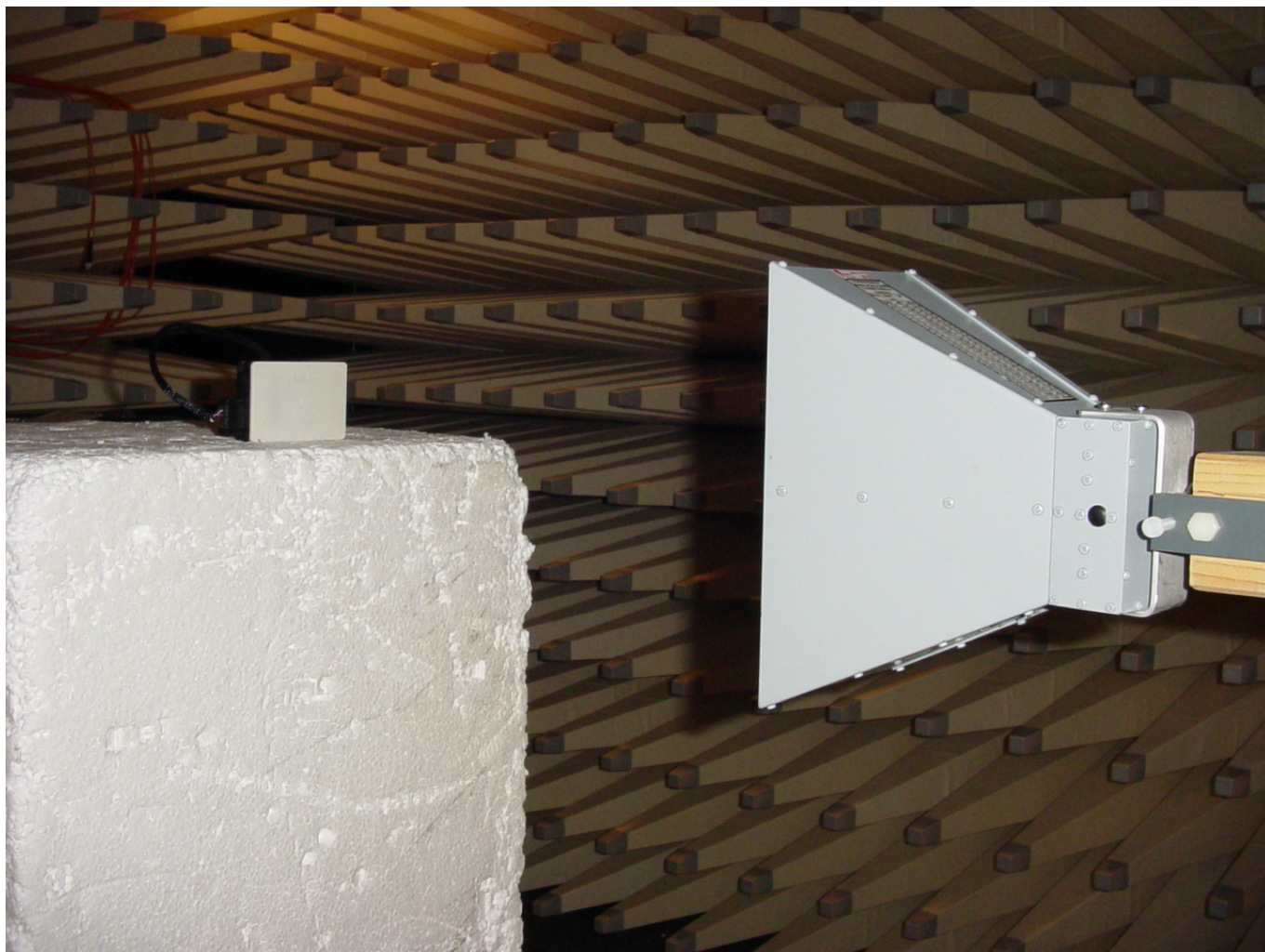
Photograph 2: Radiated Emissions Test up to 12 GHz
