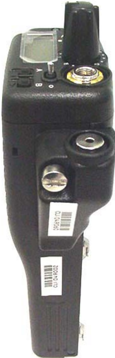
DUT with Audio Adapter Accessory (P/N: OT-V1-10430)
