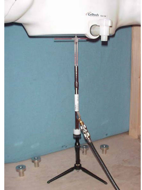
835MHz Dipole Setup
