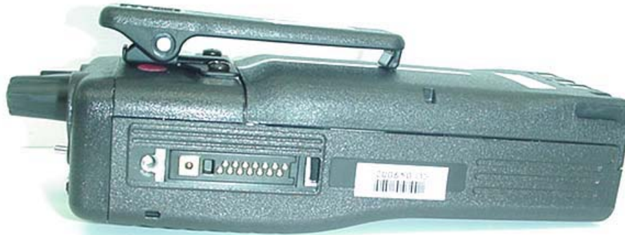
Right Side of DUT with Metal Belt-Clip & Audio Accessory Connector
