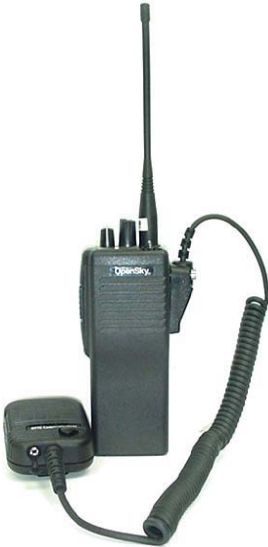
DUT with Evolution Speaker-Microphone Accessory (P/N: MC102823V1)
