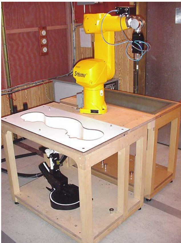
DASY4 SAR Measurement System with validation phantom
