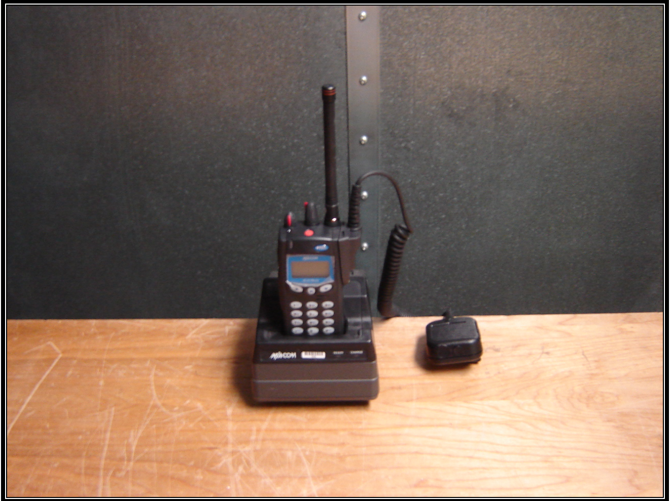
Photograph 3: Conducted Emissions – Front View
