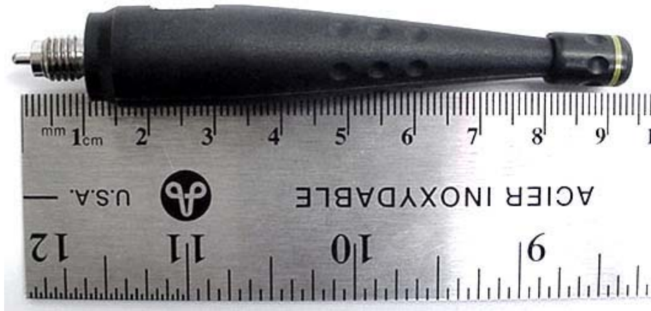
Quarter-wave Antenna (P/N: KRE 1011 1506/2)
