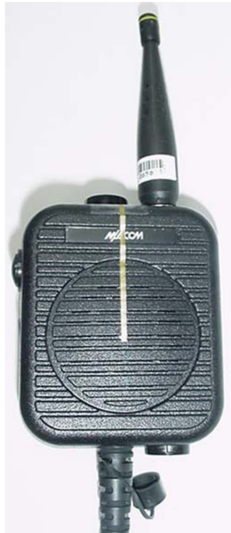
with Quarter-wave antenna (P/N: KRE 101 1506/2)
