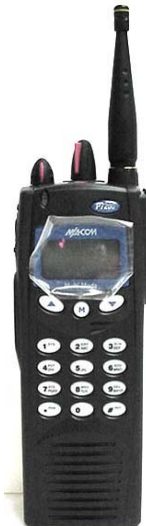
Front of DUT with Quarter-wave Antenna (P/N: KRE 101 1506/2)
