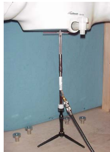
835MHz Dipole Setup
