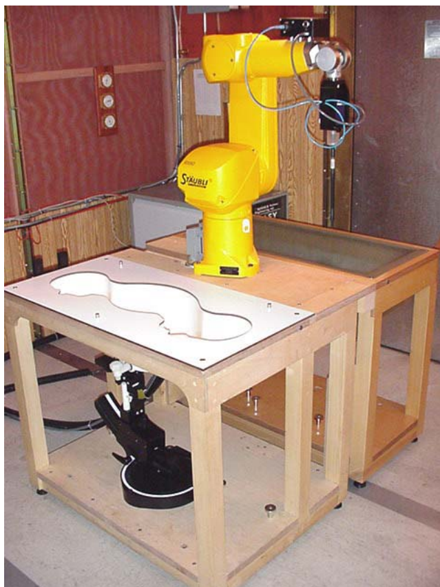
DASY4 SAR Measurement System with SAM phantom
