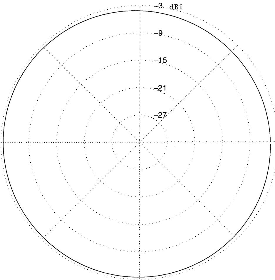
Fig. 13. The calculated radiation pattern for the horizontal xy plane for the Microphone (with nominal "1/4 wave" antenna) held in free space.
