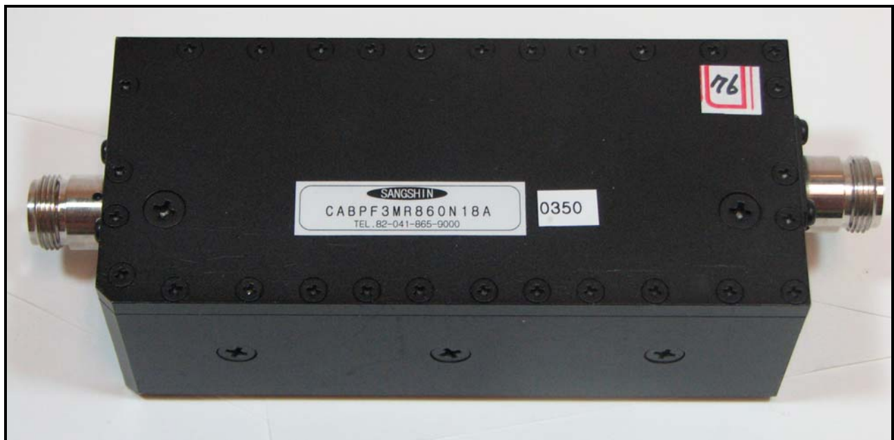
Photograph 6: HPA Output Filter
