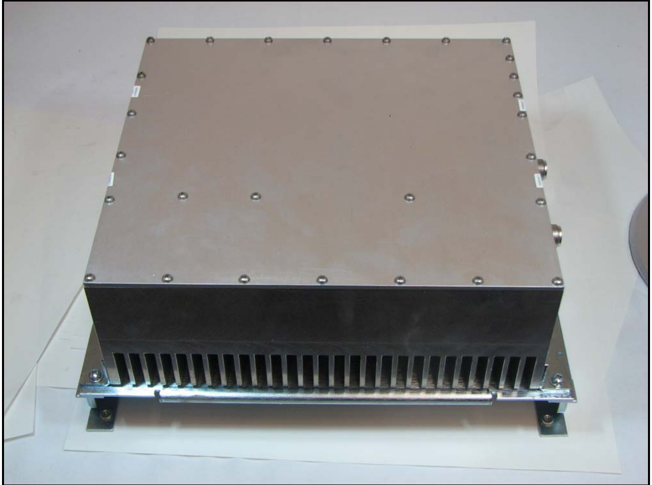
Photograph 7: HPA RF Deck Front
