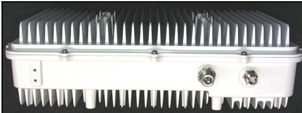
Photograph 7: RF and GPS Antenna Ports
