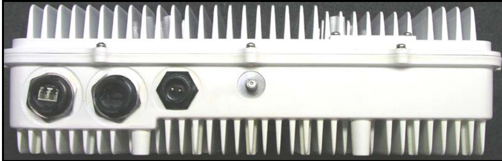
Photograph 6: Data and Power Connectors
