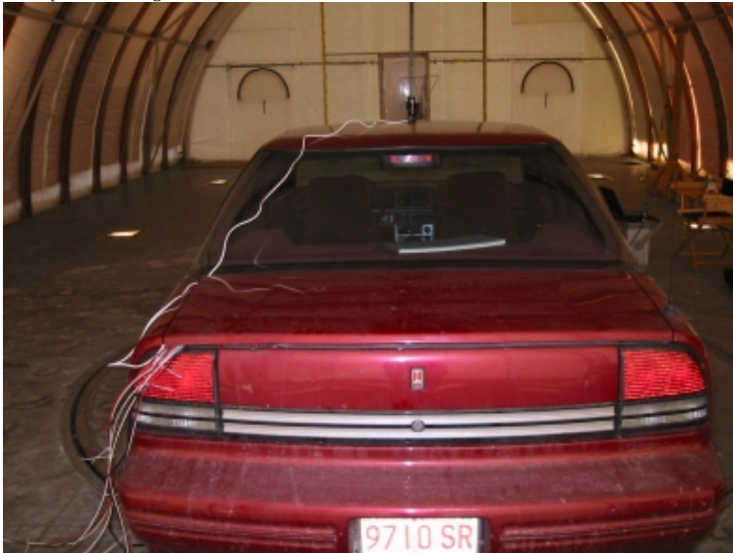
RF Exposure Testing, Roof Mount
