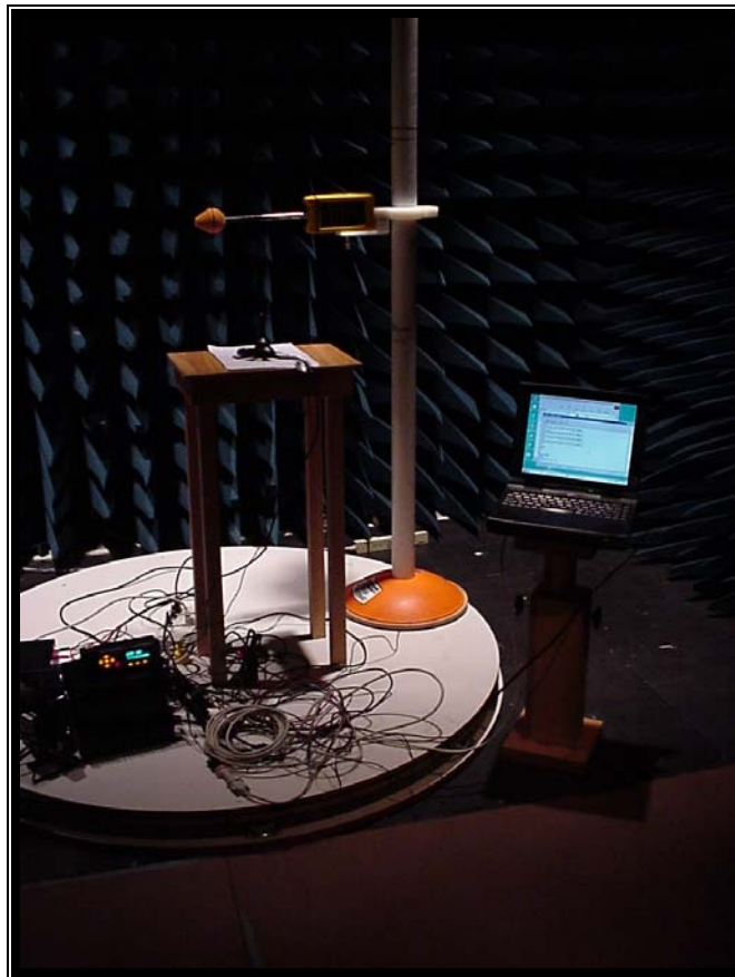
Photograph 6-1: MPE Test Setup with the Antenna in the GPS RX Antenna Base
