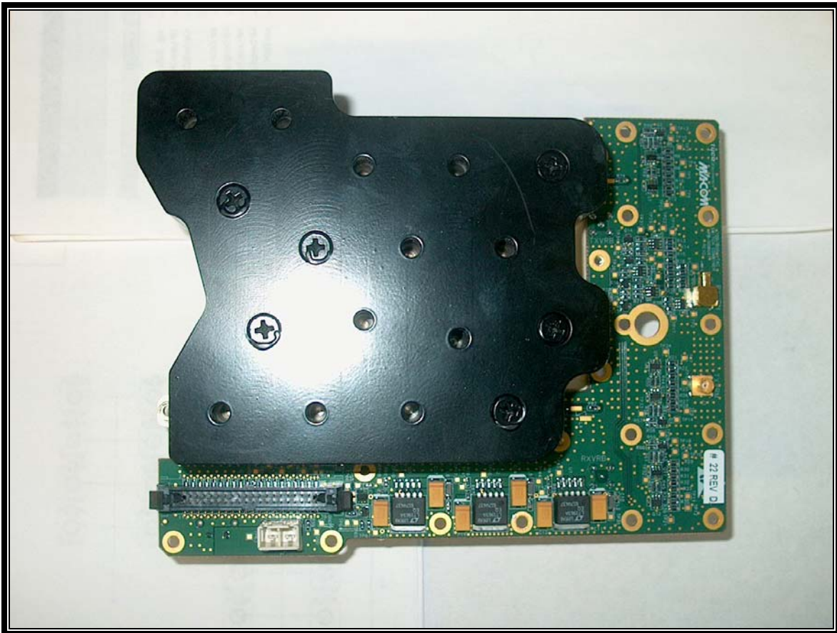
Photograph 14: RF Switch Combiner Board + Triplex Filter Top
