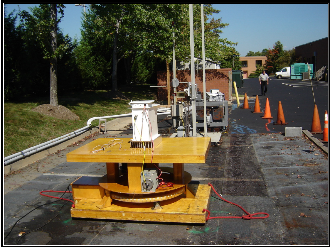
Photograph 3: Radiated Emissions - Front View
