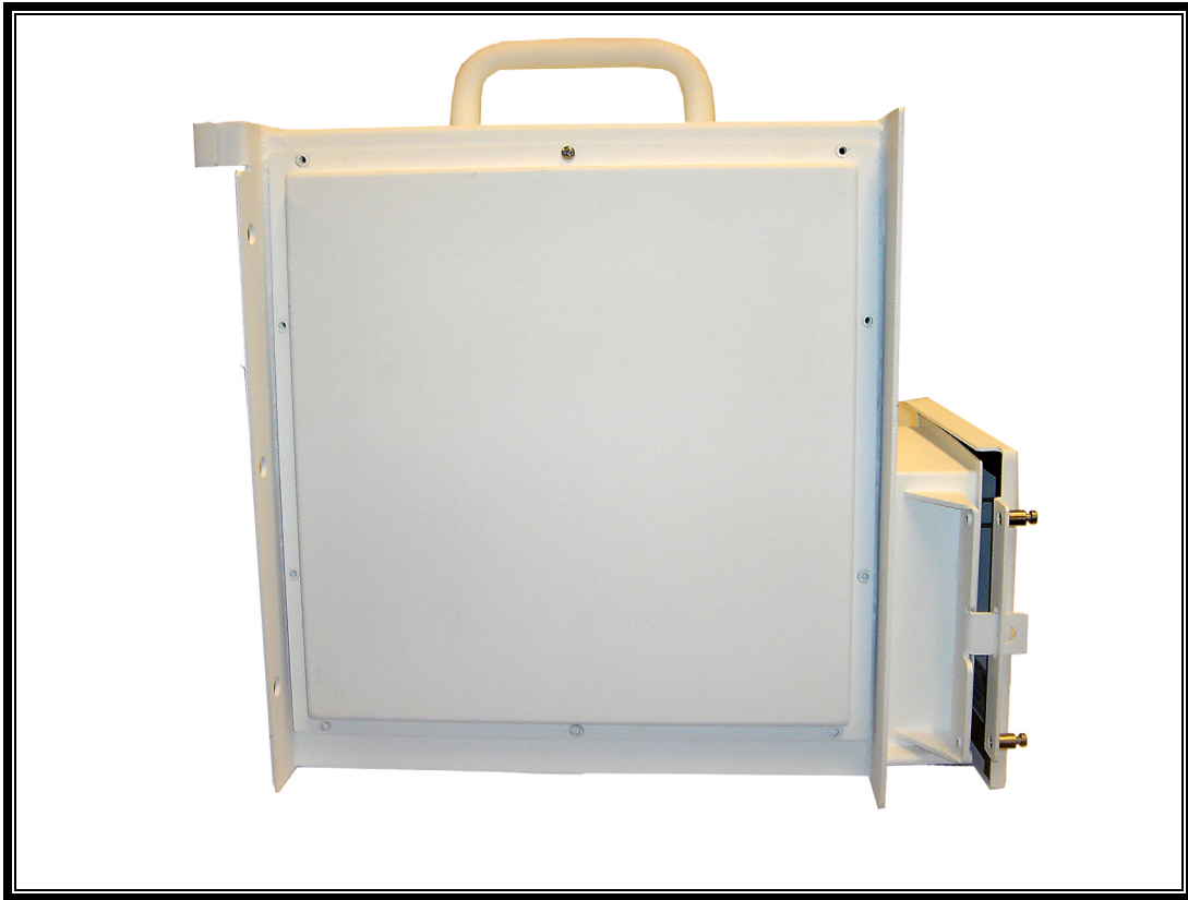
Photograph 7: 700 MHz Cell Site Enclosure Side View 1
