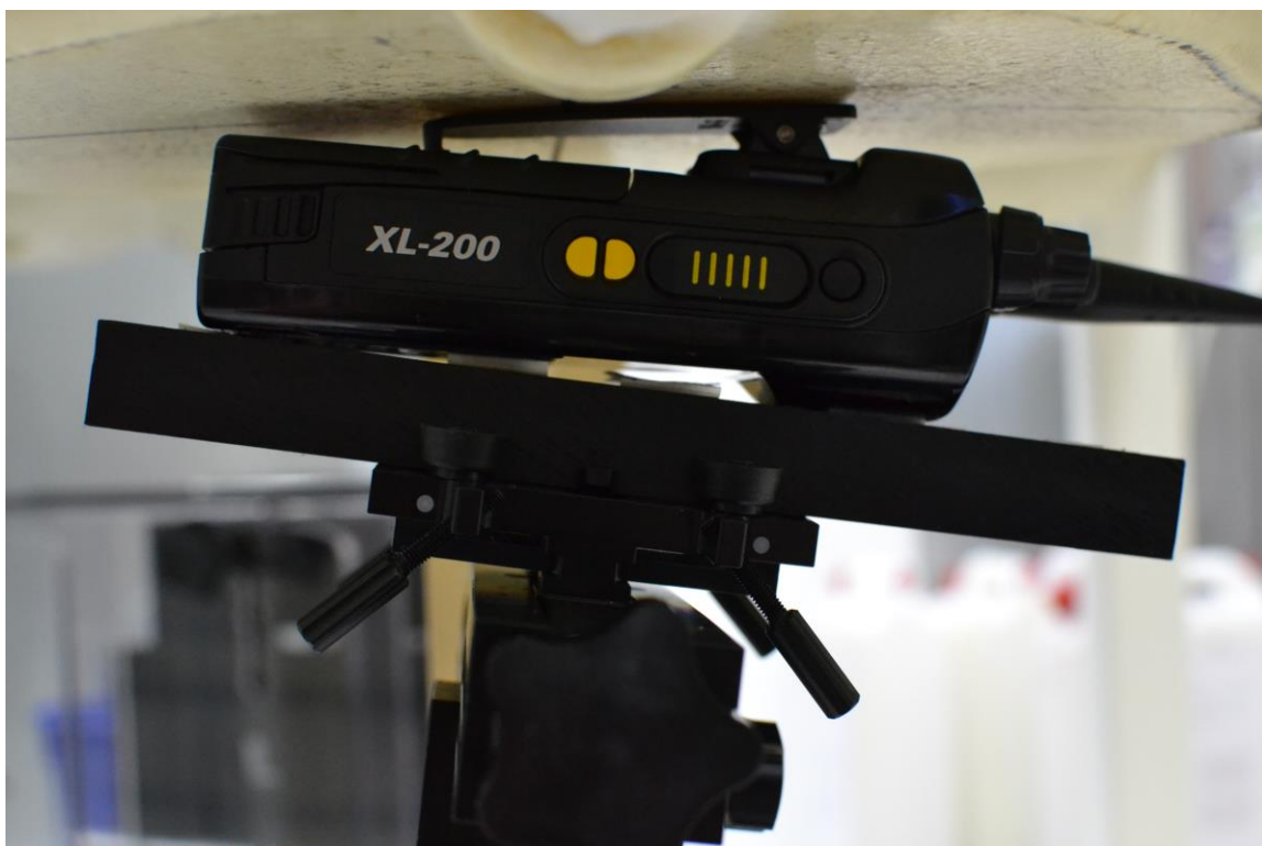
SAR Test Setup Photo 2 – BW Grouping 1 Test Distance
