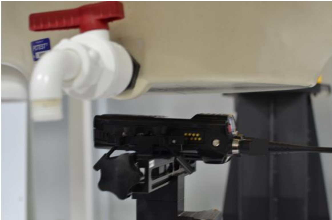
SAR Test Setup Photo 1 – Head Testing at 2.5 cm
